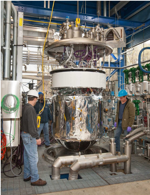
Figure 2. Reduced boil-off test article.
