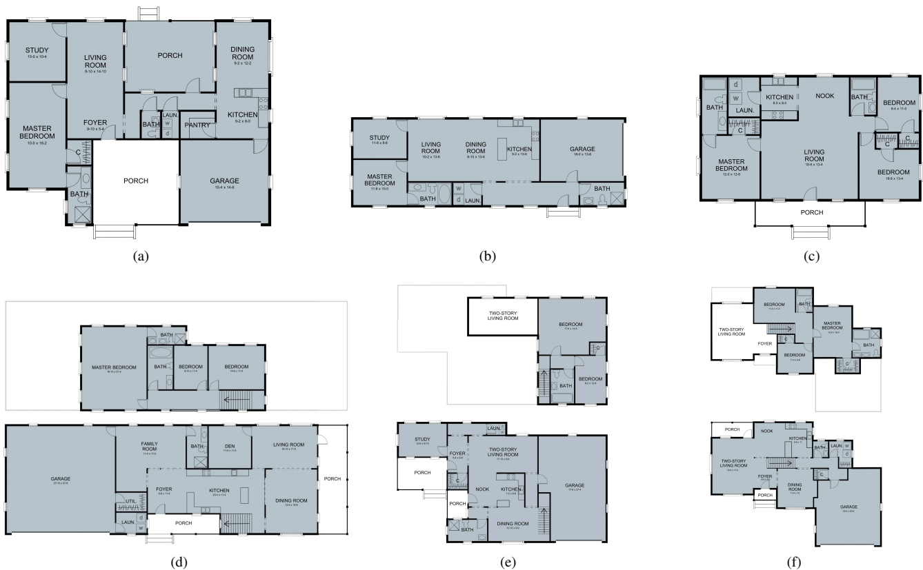
Figure 13: (a,b,d,e) Computer-generated building layouts. (c,f) Real-world layouts, reproduced from a catalogue, shown for comparison. The bottom row shows two-story layouts.
