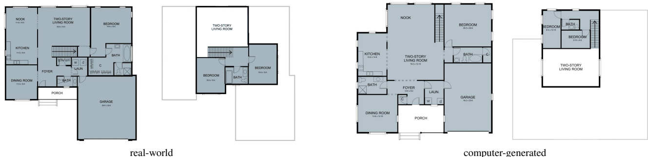
Figure 12: A two-story layout designed by an architect (left) and an automatically generated layout for the same architectural program (right).
