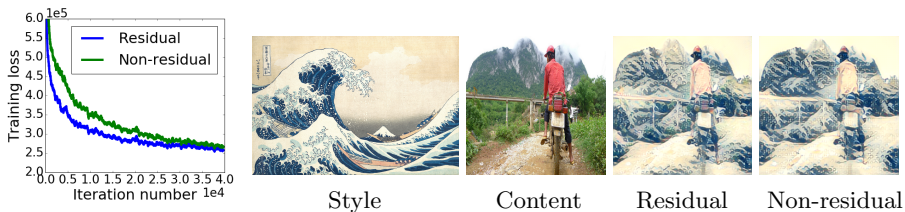
Fig. 2. A comparison of residual vs non-residual networks for style transfer.
