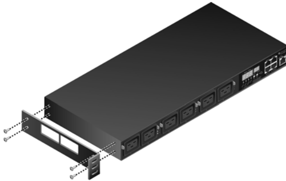
Figure 2.1: Attaching Mounting Brackets to a Horizontal PM PDU
