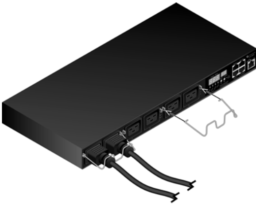
Figure 2.3: Attaching Retention Clips for a 6-port Horizontal PM PDU
