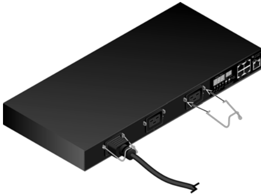
Figure 2.2: Attaching Retention Clips to a 3-port Horizontal PM PDU
