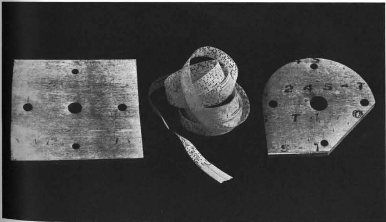
SAMPLE PRODUCT of the automatic machine tool described in this article is the cam shown at right.
