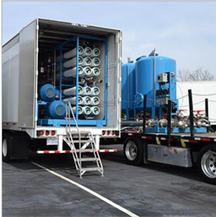
Figure 8-7. Trailer Mounted Mobile Water Treatment System
