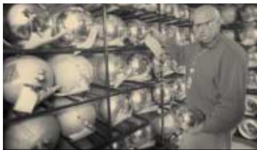
Dr Paul Frazer decants a sample of air taken from the Cape Grim outpost on the southern tip of Tasmania as part of an international project to monitor CFCs in the atmosphere and the Ozone layer.
