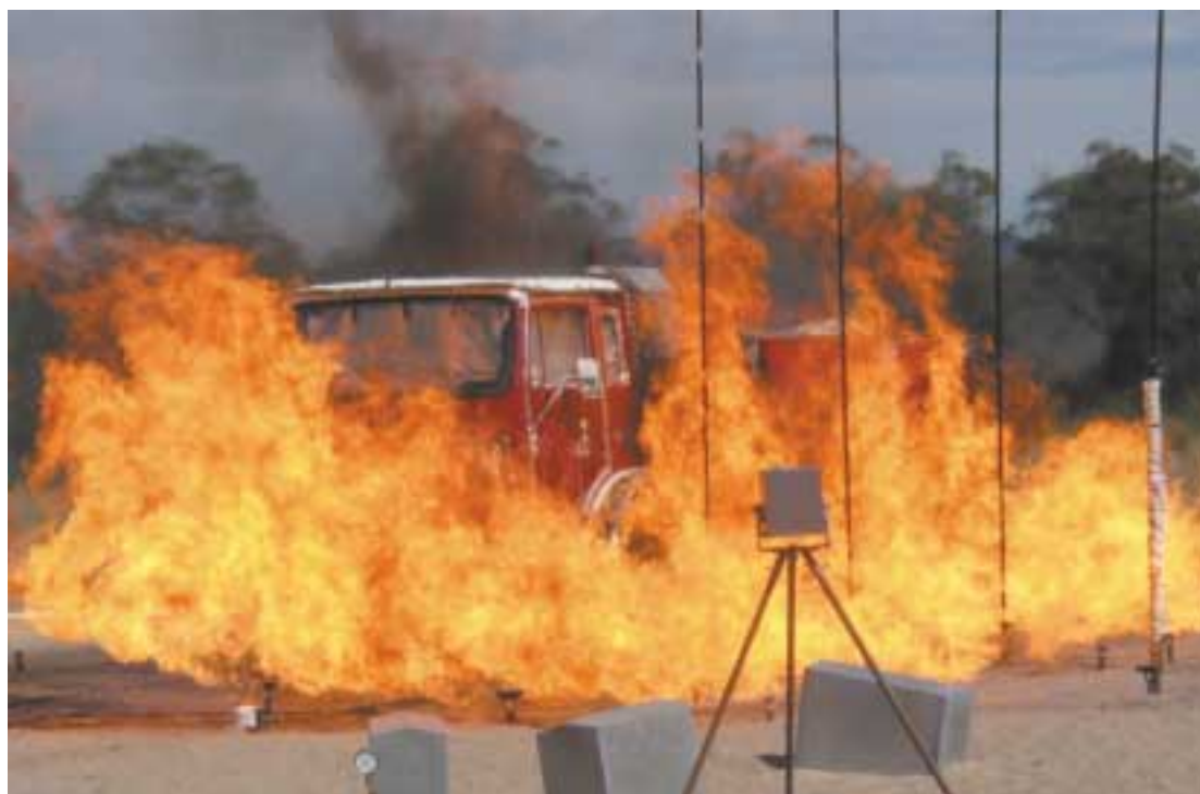
In a world-first, NSW Rural Fire Service and the Country Fire Authority of Victoria, working with CSIRO researchers, have developed and proved a new fire truck protection system which will help fire fighters survive being caught in a bush fire. Photo: Nathan White. CSIRO Manufacturing and Infrastructure Technology
