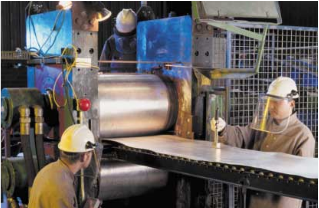
Australian scientists at CSIRO have developed an industrial-scale pilot plant, which is now producing near-net-shape, or close to product thickness, low-cost magnesium sheet. Photo: Mark Fergus, CSIRO Manufacturing and Infrastructure Technology
