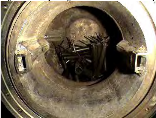
Figure 3-8: SDC Chamber with 20 Simulated Open Fin NCRM Sections Loaded
