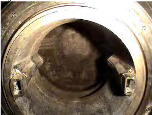
Figure 3-9: Empty SDC After One Dump Cycle (Simulated NCRM with Fins)
