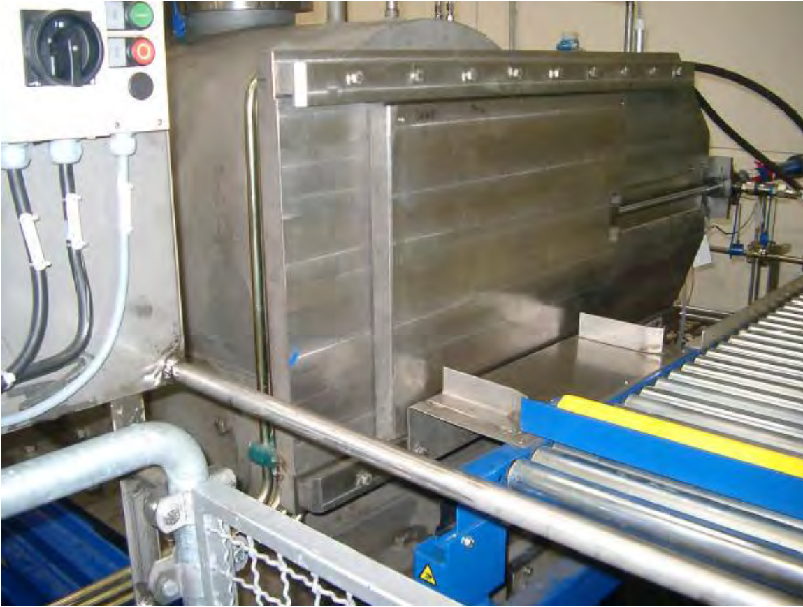
Figure 2-6: First Loading Door Closed and Sealed
