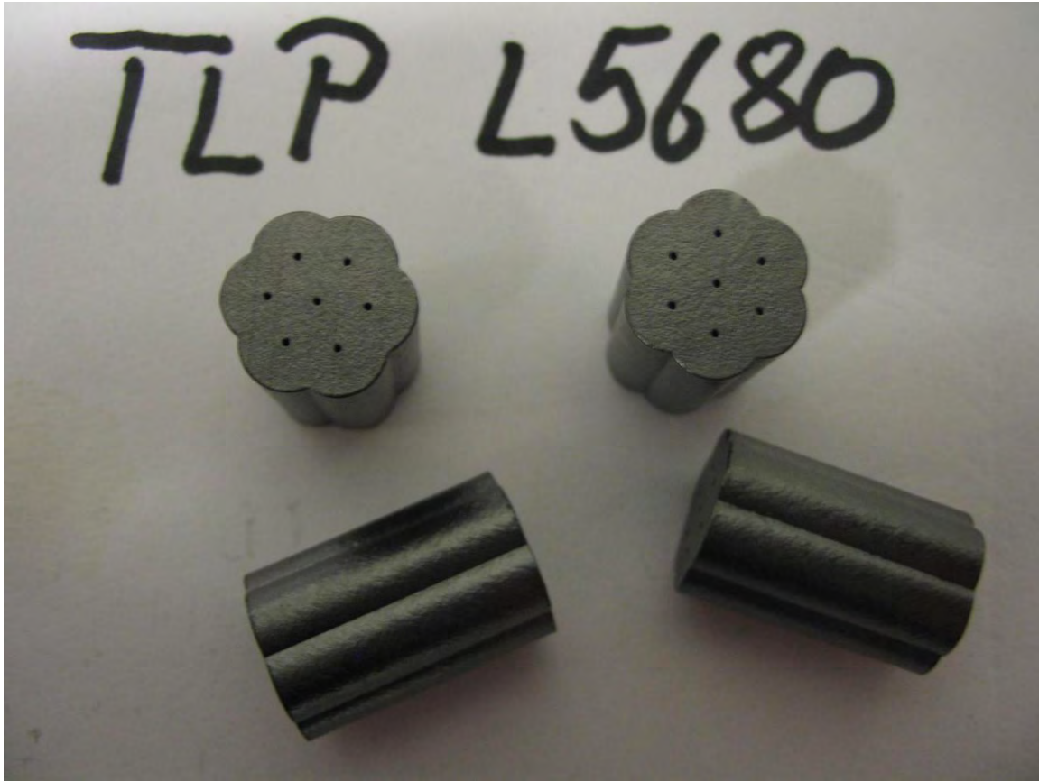
Figure 4-9: Configuration of the Propellant
