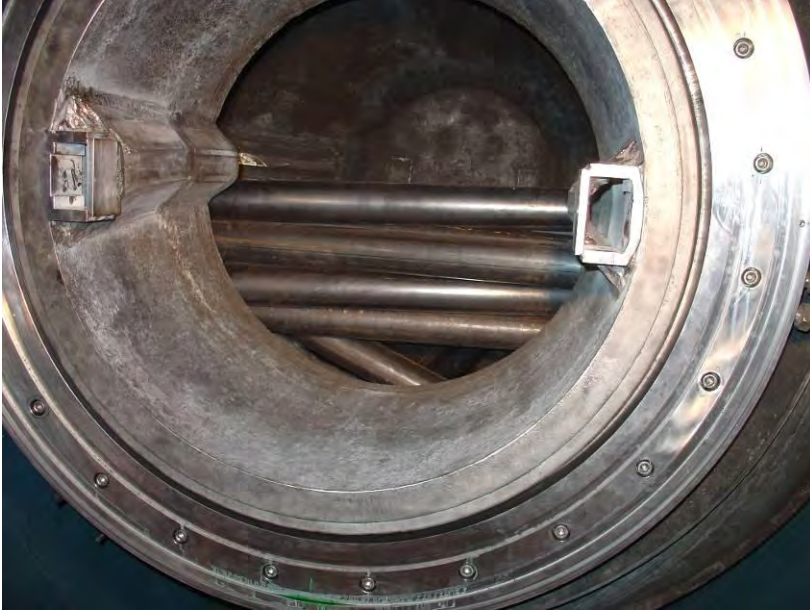
Figure 4-22: Bridging After First Rotation in Run 1
