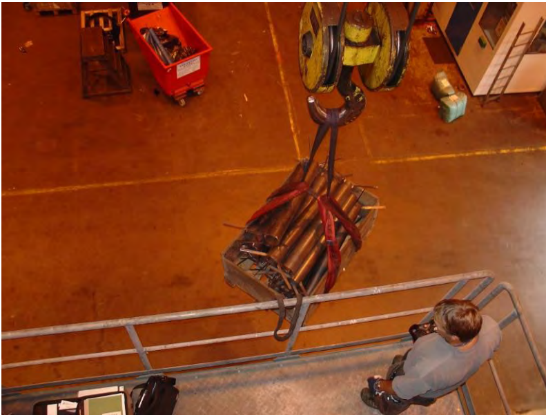
Figure 4-27: 20 Finned Tubes Being Lifted in Preparation for Run 3
