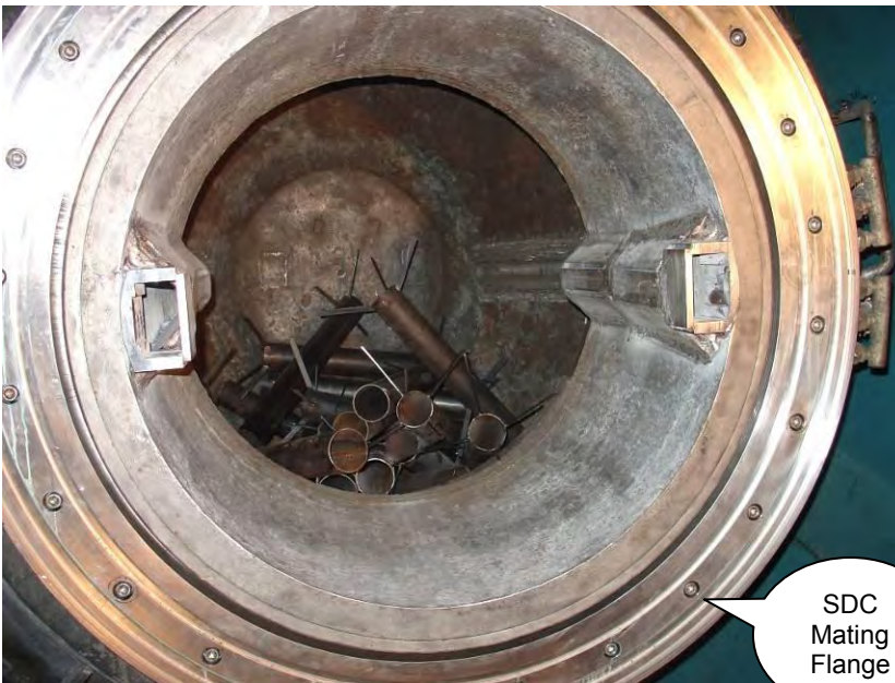
Figure 4-25: SDC Vessel Loaded with 20 Finned Tubes
