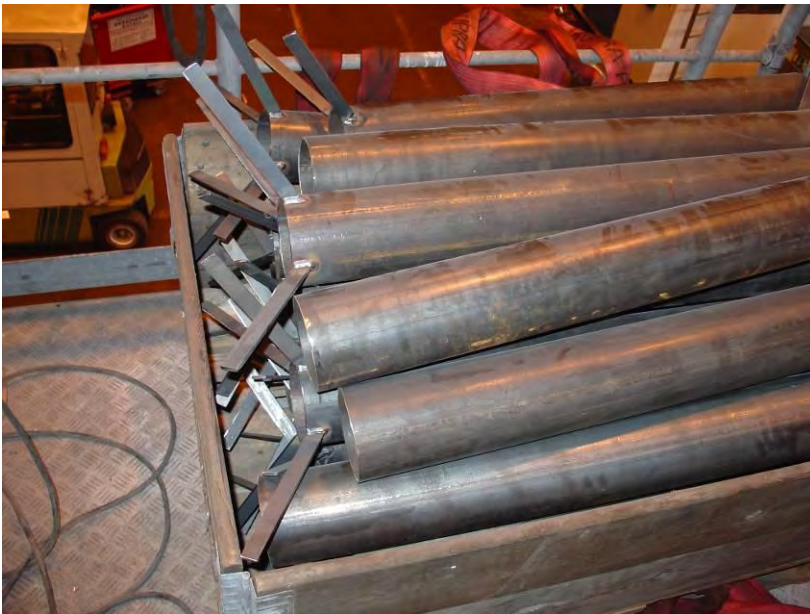
Figure 4-23: Simulated Rocket Motor Casings with Fins
