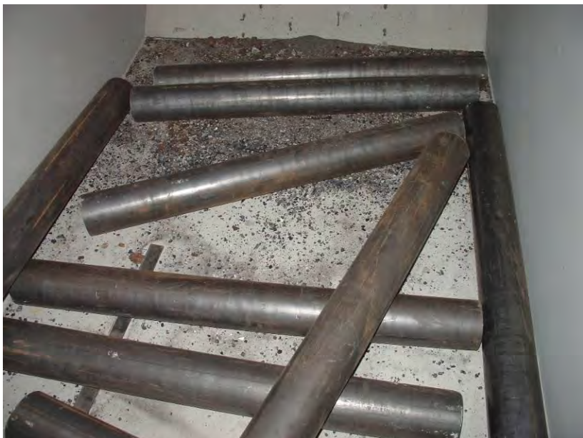
Figure 4-21: Nine Straight Tubes in Scrap Bin after First Rotation
