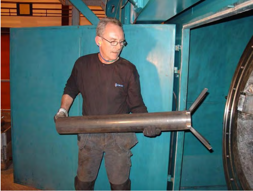
Figure 4-24: Finned Tube being Loaded into SDC Vessel
