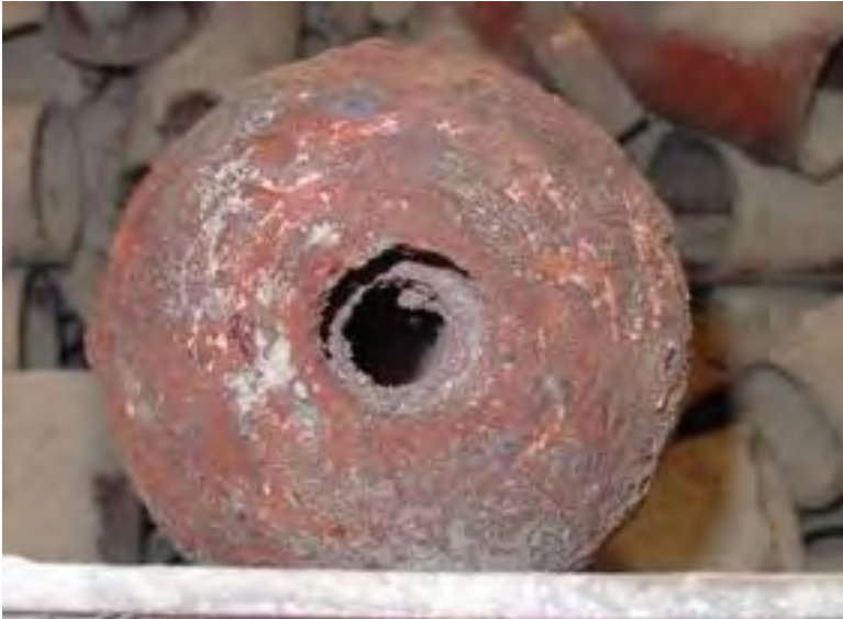
Figure 4-6: Treated 10 cm Projectile with Nose Plug Blown Out
