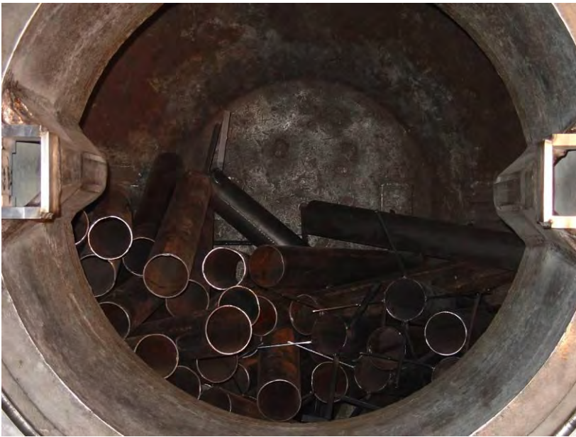
Figure 4-29: SDC Vessel Loaded with All 50 Tubes for Run 3
