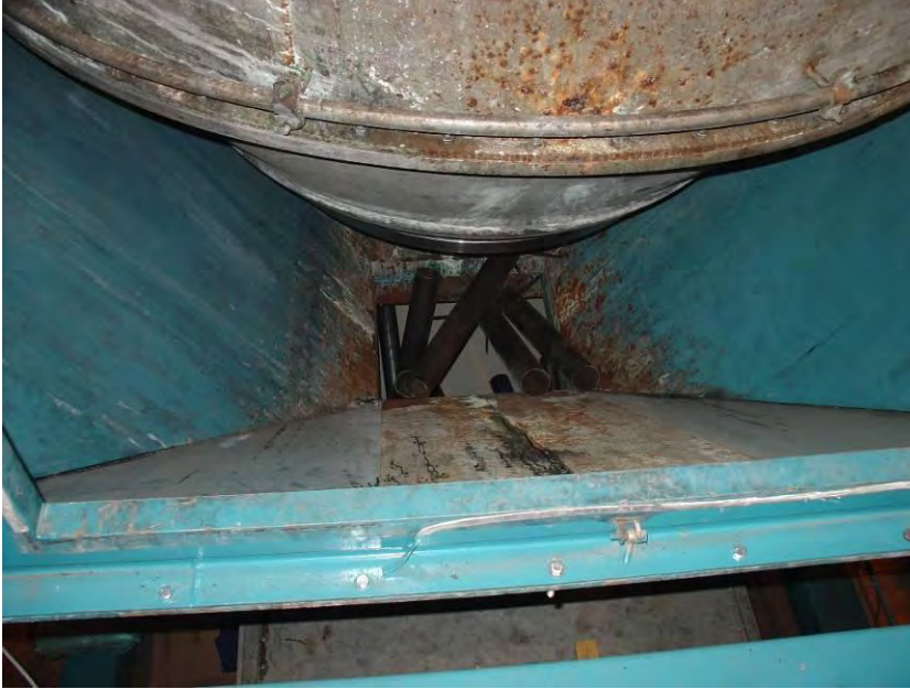
Figure 4-26: Finned Tubes Bridged Across Discharge Chute Funnel
