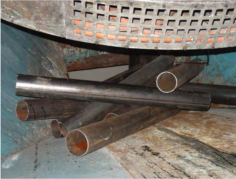
Figure 4-30: Tubes Bridged in Discharge Chute after Run 3, Rotation 1
