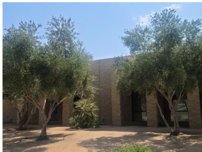
Trees along the west facing side of buildings shade windows and walls from direct sun. Palm Desert City Hall
