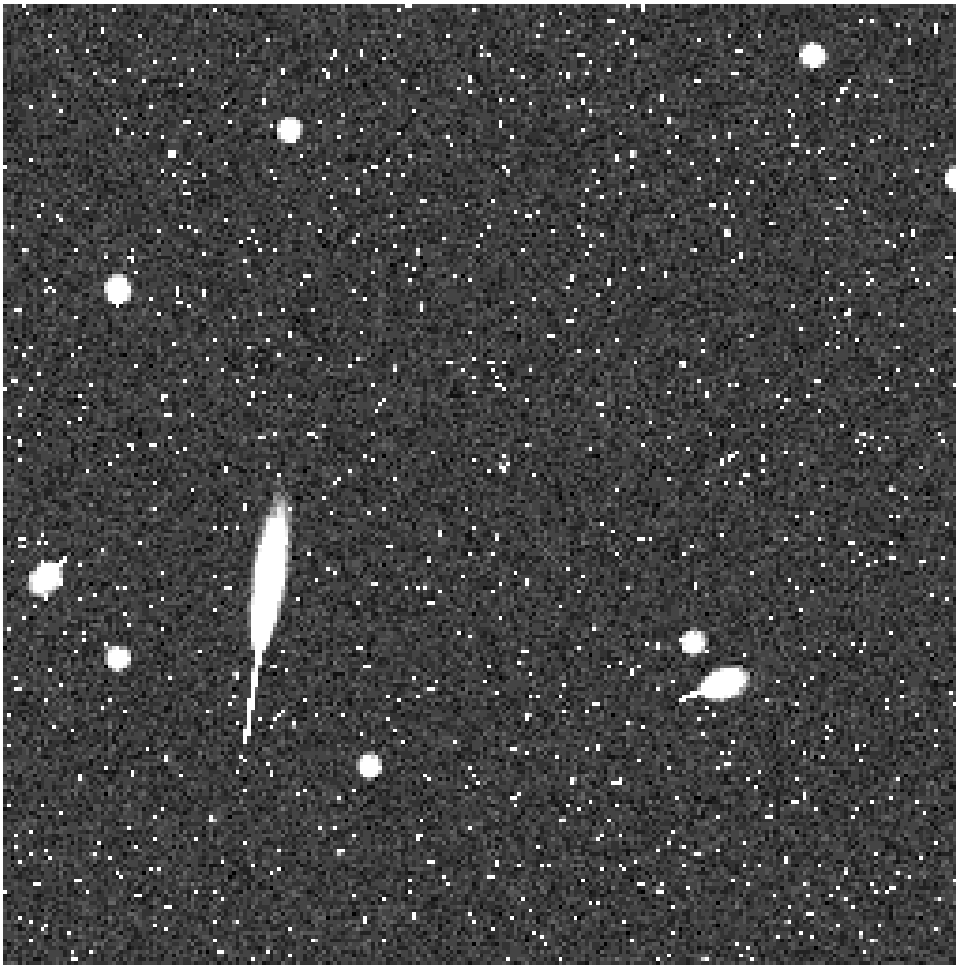
Figure 7.2: Example of a simulated front-illuminated CCD frame, containing 1000 1keV photon events and 10 particle events
