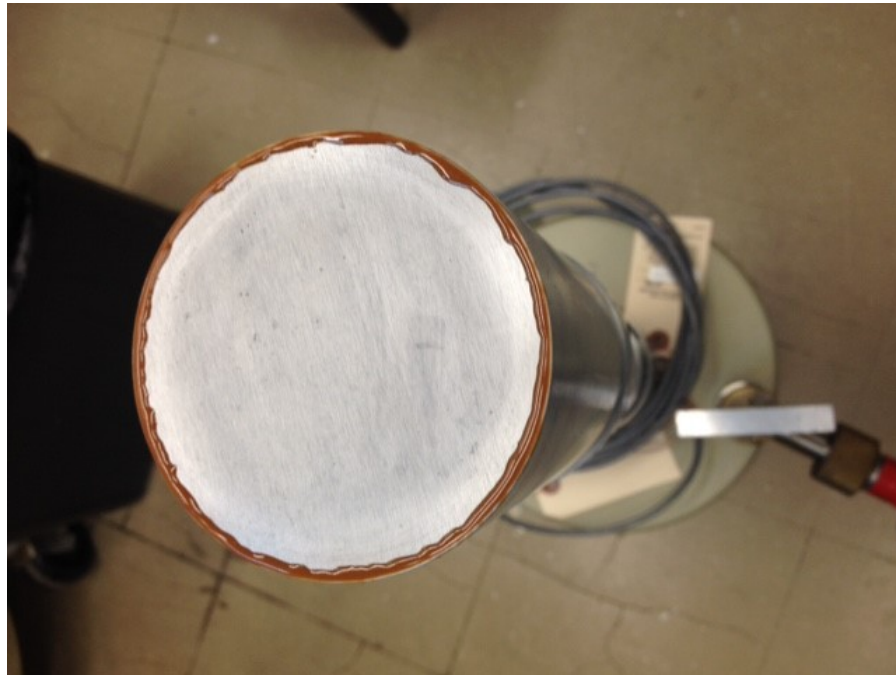
FIG. 1. Externally patched epoxy seal of the Be window in early 2017.
