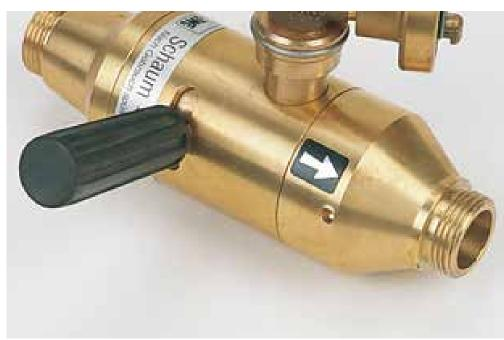
Manufactured from solid brass by AWG in Germany, this inductor can be mounted inline (adjustable) or in a by-pass set up (fixed) between the HP pump outlet and HP hose reel drum inlet to produce an effective foam media.
