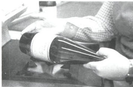
Bar code being read by laser.
