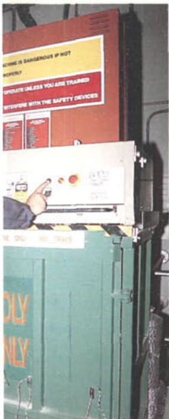
David Lamphee, in-store cleaner at Hedge End, uses the baling machine which prepares waste packaging for recycling.
