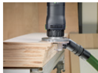
Chamfering plastic or solid wood veneer.
