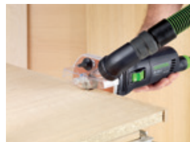
Flush trimming of plastic or solid wood veneer.
