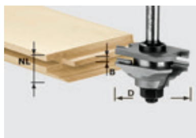
Profile/spring cutter HW with ball bearing guide, shank 8 mm HW s = 8
