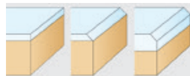
Flush Chamfered Flush + chamfered
