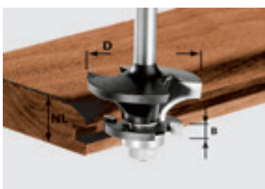
Counterprofile cutter groove HW with ball bearing guide, shank 8 mm
