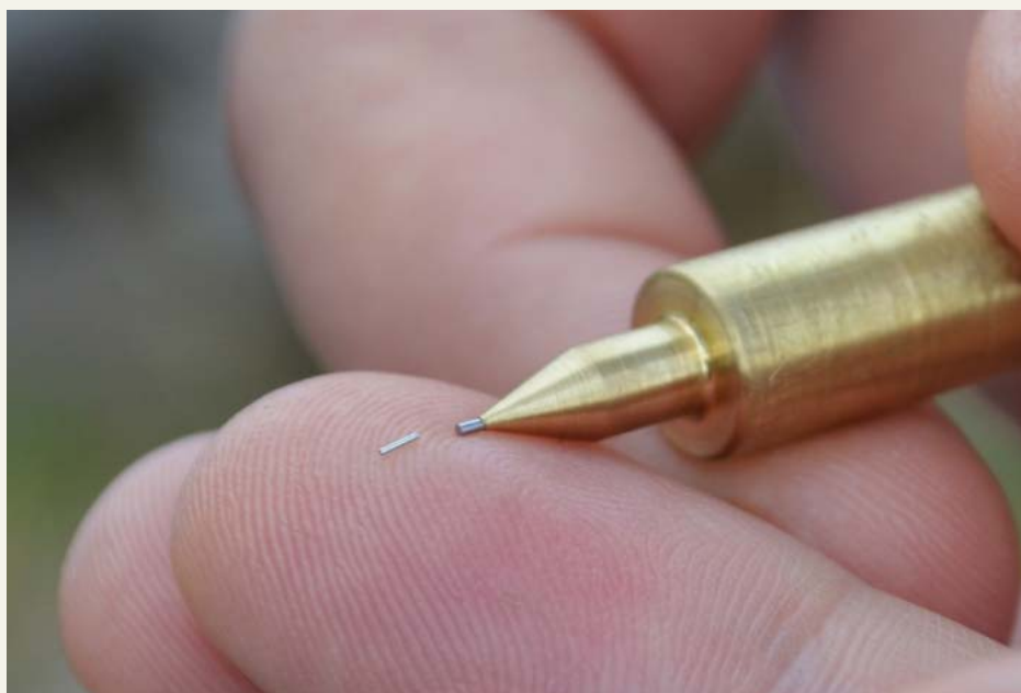
Magnetic tag that allows tracking the migration routes and breeding areas of sturgeons.
