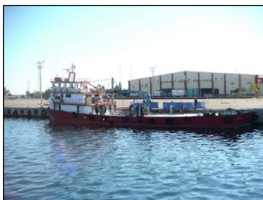
TS1: a ship with length 45m made of sheet iron. Berths 20 persons. Crane for 20tons, tank with 4 cooler systems and freezer. Also the generator and ice machine (providing ice from sea water)
