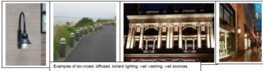
Figure 14.195-20: Downward and Diffused Lighting, Wall-Washing Lighting
