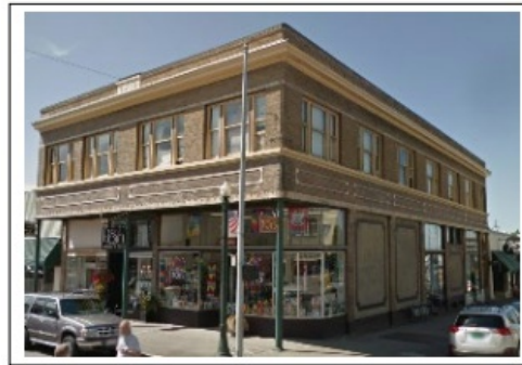
Figure 14.115-2.b: Base, Middle, Top of Building
