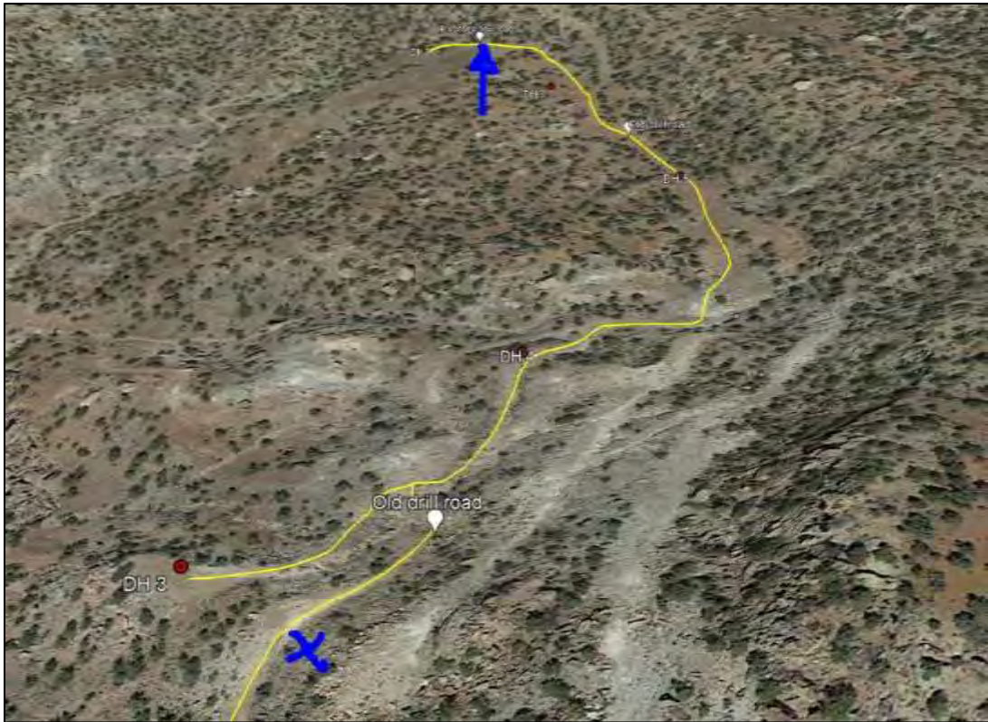
Figure 13: A screen capture of a google earth image showing the locations of drill holes SDH3 to SDH7. The previous photo of SDH3 was taken at the blue X. SDH3 could be relocated to the X location and eliminate ~200 feet of disturbance. The blue arrow shows where SDH7 could be placed to avoid disturbance on relatively erodible aeolian soil.
