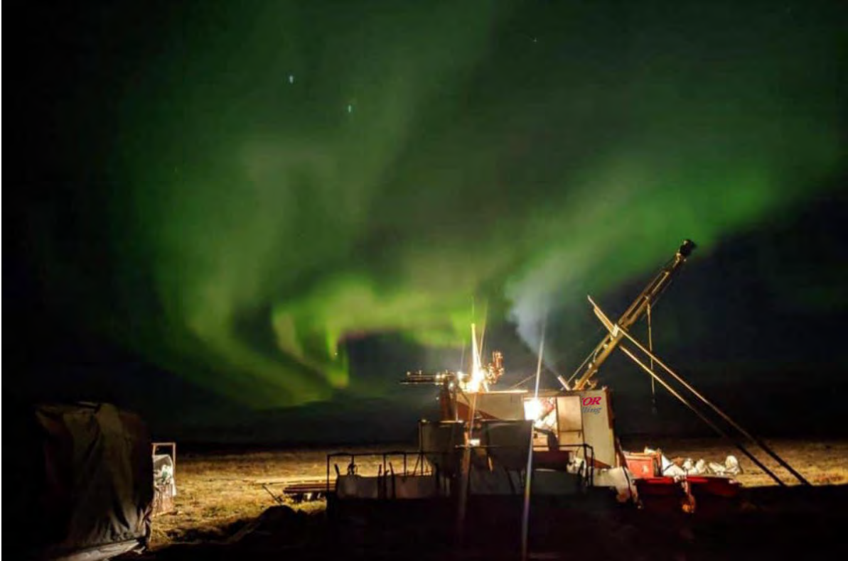
Figure 1 – Examples of drill rig down lighting used for nighttime drill projects. A secondary trailer light plant/generator may also be used to illuminate the drill pad to ensure safe operations.
