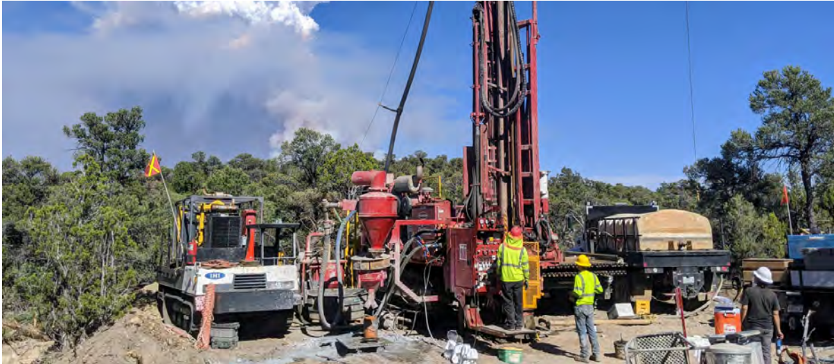
Figure 1 – Example drill rig setup with support equipment (rod tray, compressors, and water truck) from a separate 2020 drill program.
