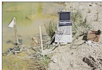
in situ: cages with chambers, battery-operated MFB and laptop
