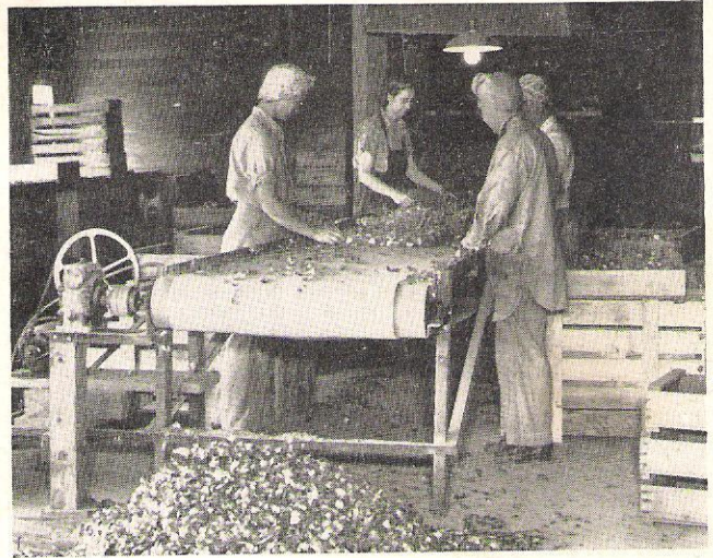
Grading Daffodils from a moving belt after going through a shaker which cleans them.
