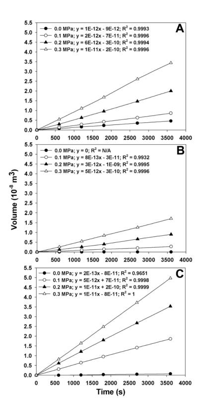
**Figure 3.5** Steady-state water flow per unit root surface area with an increasing driving force (i.e., induced hydrostatic pressure changes). This graph displays typical results. Legend inset in graph.
