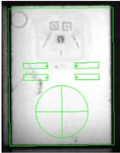
Figure 15: Teaching the OSIRE® E4633i into the ASM Siplace Vision System
