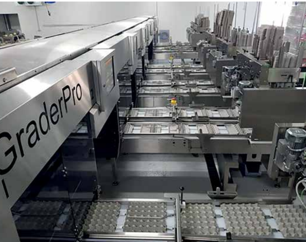
World's largest grading machine sorts and packs eggs into consumer egg packs. Millions of eggs end every day in supermarkets all over the world
