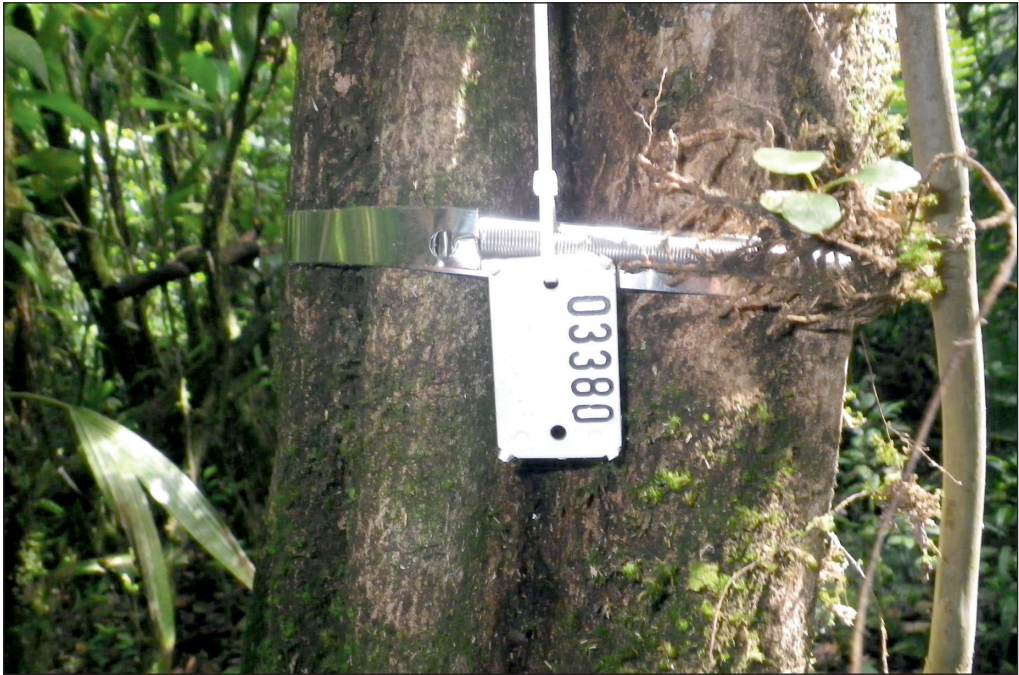
Figure 2. Tape dendrometer and label attached to the tape.
