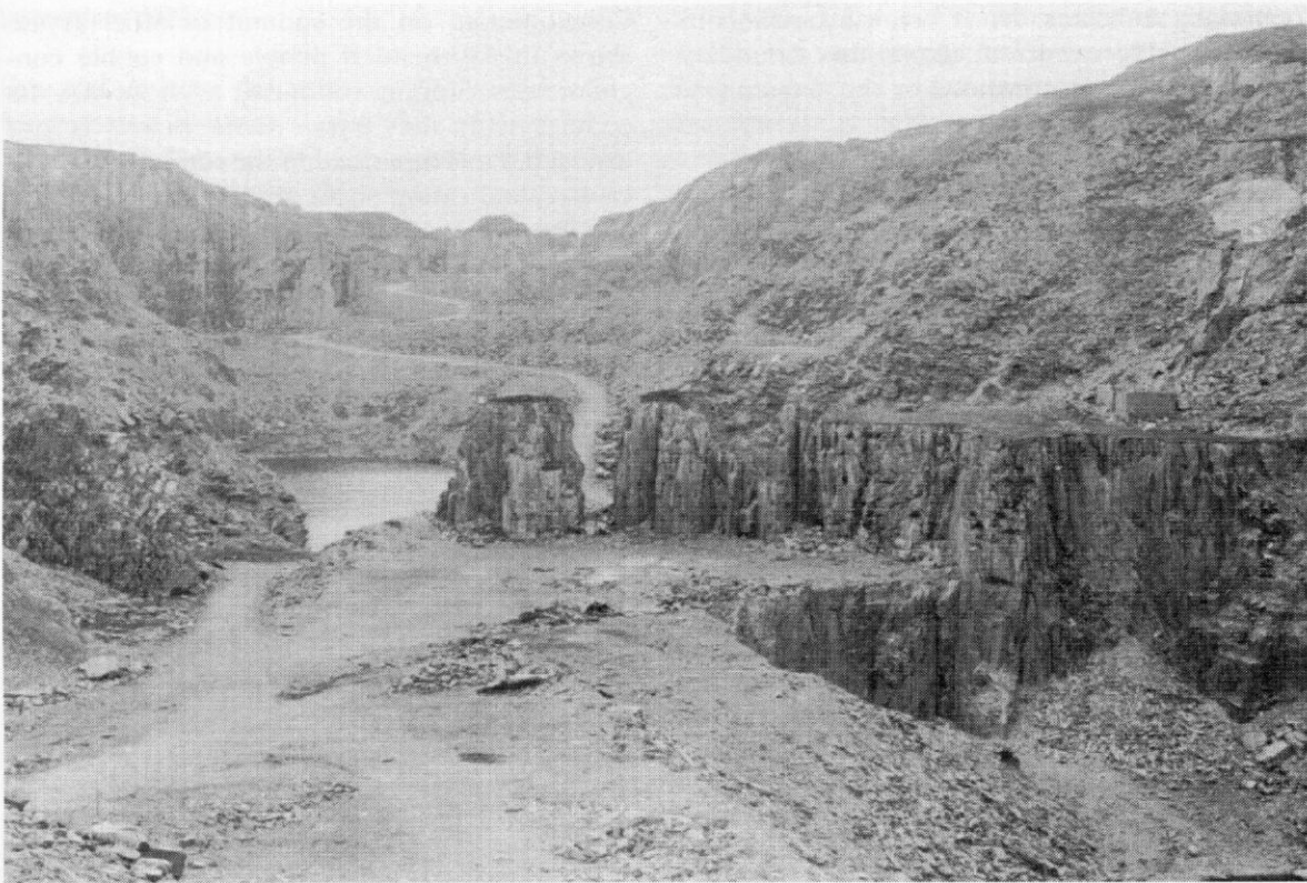
Figure 3.14 Alexandra Quarry, Moel Tryfan, looking south-west, showing vertically cleaved Llanberis Slate dipping at about 45^\circ to the left. The Dorothea Grit to the right does not show the cleavage conspicuously. (Photo: British Geological Survey photographic collection, L2333.)
