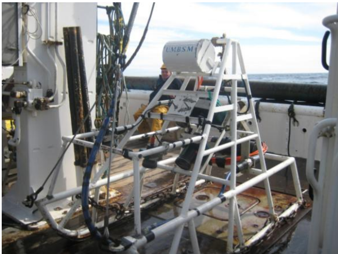
Figure 2.7 Drop down sledge video and camera system employed during MPA search feature and Priority Marine Feature (PMF) surveys undertaken by HWU with Marine Scotland Science off Noss Head, north-east Scotland (Hirst et al 2012; equipment loaned from University Marine Biological Station, Millport).
