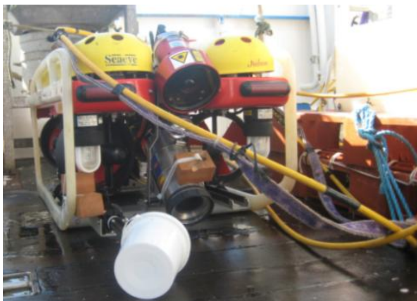
Figure 2.8 ROV Seaeye system used by HWU / Marine Scotland Science during the PMF and MPA search feature validation surveys carried out off the north-east coast of Scotland in 2011 (Hirst et al 2012).
