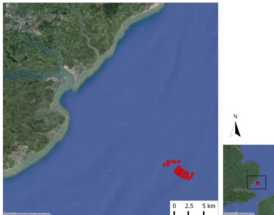
Figure 4.6 Chart showing the distribution of co-located 0.1m 2 Hamon grab samples and seabed images collected across the Cutline site between 2008 and 2010. Note that although seabed images were taken at the same sampling stations as the grab samples they were taken at different times during the survey and will not be exactly co-located. Precision of co-location estimated to be <10m.
