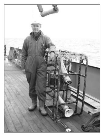
Figure 2.1. The "bed-hop" camera system in its supporting grame, just prior to deployment over the side of a research vessel.
