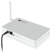
Stretch 2.0: controls the Plugwise system.
