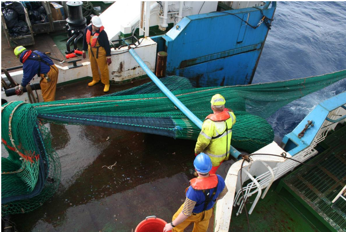
Figure 4.1: The trawl comes aboard with the three ground bags attached under the ground gear (the main cod-end trails behind and is still in the water). Photo FN.
