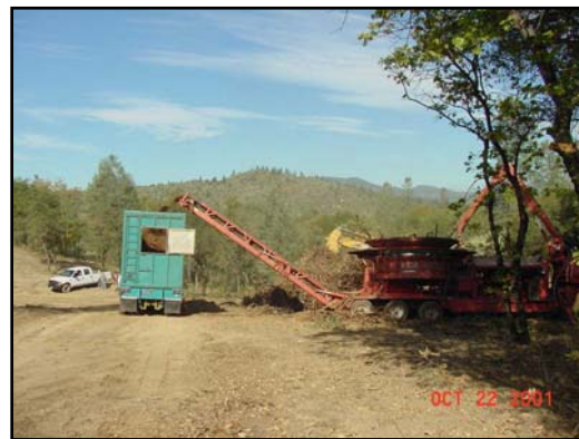
Biomass Collection in Action. Tub grinder on right. conveyor takes biomass into the
