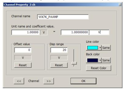
It is possible to display in engineering units by applying coefficient to a voltage that is input to the input connector.
