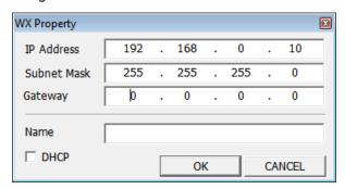
Click the OK button to apply the IP address parameters for the WX-7000 series. It is not necessary to restart the WX-7000 series. It takes a few seconds for the changed settings to actually take effect. So, wait at least 5 seconds and then connect to the WX-7000 series. If the list is not updated or the entry disappears from the list, click the Update List button to update the list.
