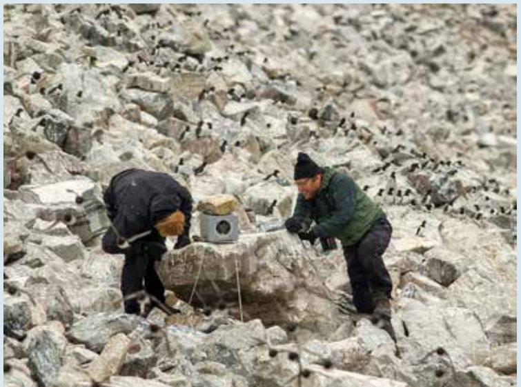
Figure 1. Mounting a still camera in a weather proof box on top of a boulder in the Paakitsoq little auk colony. The camera took a picture every hour from mid-April to early September. (Photo P. Lyngs).
