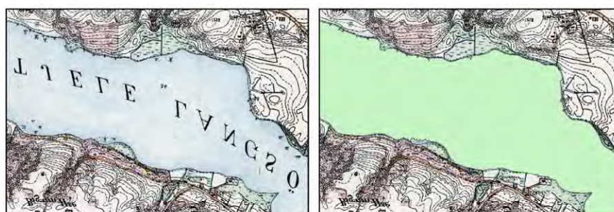
Figure 3.10 Illustration of text (place names) overlapping a map theme (water body) colouration (left) and the associated completed mapping of the water bodies (right).
