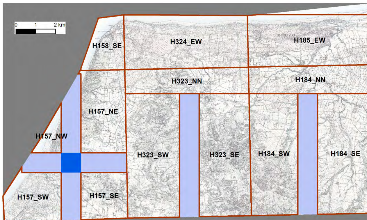
Figure 3.4 The map sheet parts applied for the Hirtshals study area, with 2-way overlaps shown in light blue and a 4-way overlap shown in dark blue.
