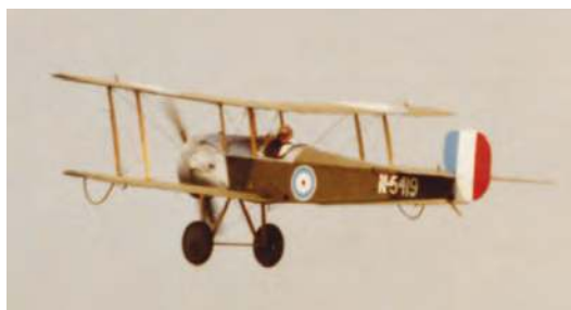
Figure 1. Leo Opdycke flying his Bristol Scout over Rhinebeck, New York: first flight, 1983. Leo built this aeroplane as a reproduction of the original 1914 Bristol Scout D with an original LeRhône rotary engine. Photograph by Bill Hammond. Collection of Leonard E. Opdycke.
