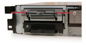
Squeeze the tabs gently and swing the tray latch upward.
