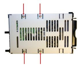
To remove the hard drive from its cage, set the assembly on a soft surface and remove these four screws.
