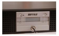
Pull on the right hand side of the front panel to remove it.
