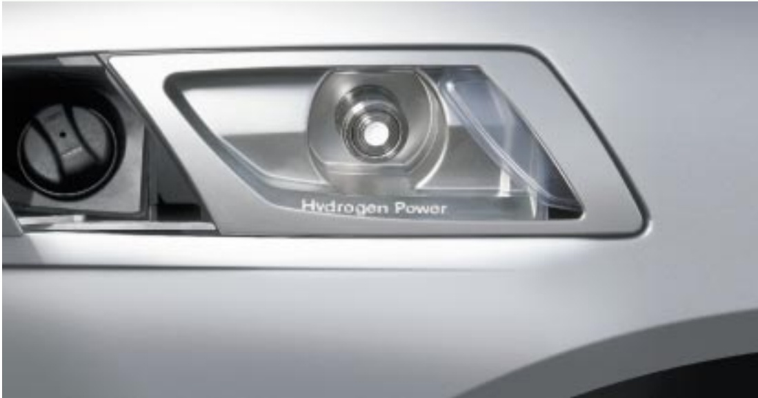
The BMW 745h prototype based on the new 7 Series with both a hydrogen and a petrol tank.
