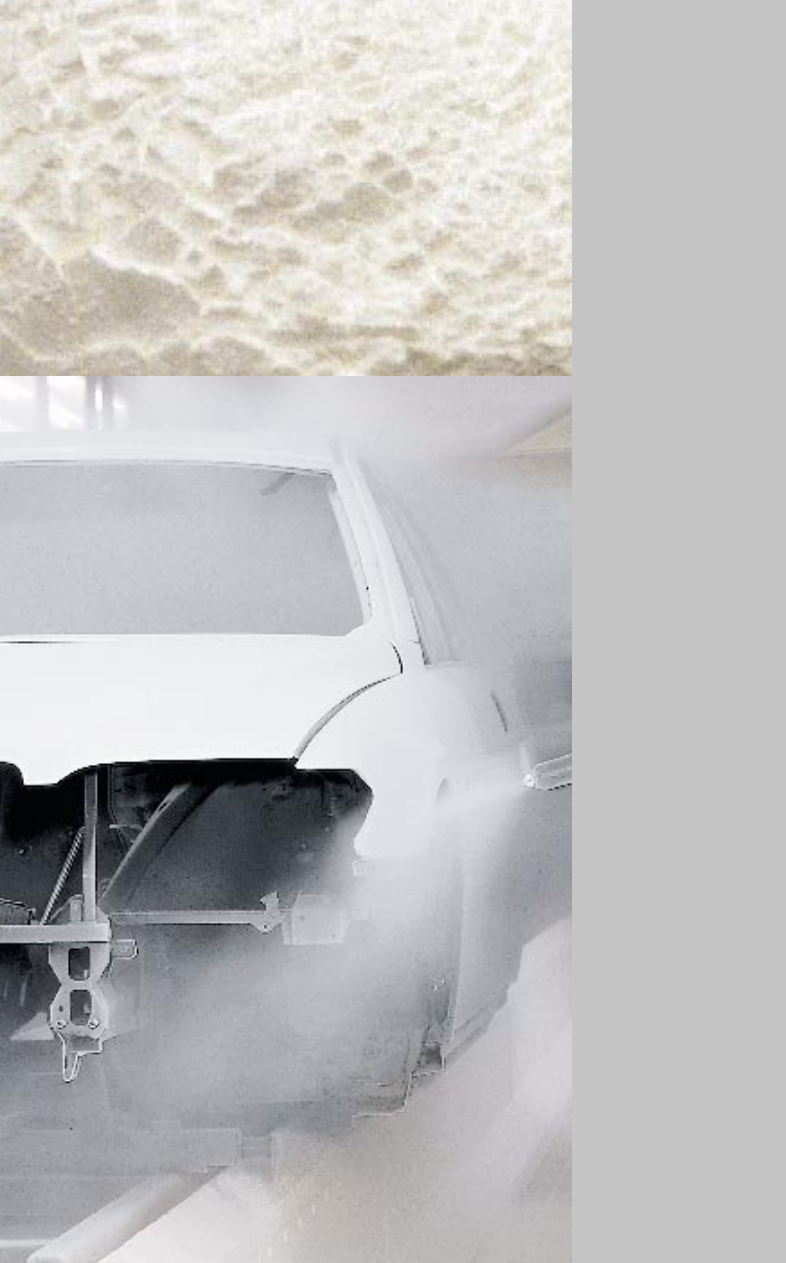
[1] Powder clear coating – BMW 7 Series production at the Dingolfing plant
