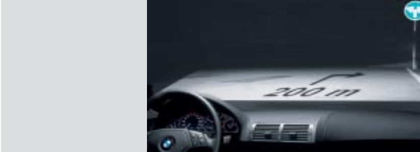
BMW pixel headlight: navigation instructions projected onto the road
