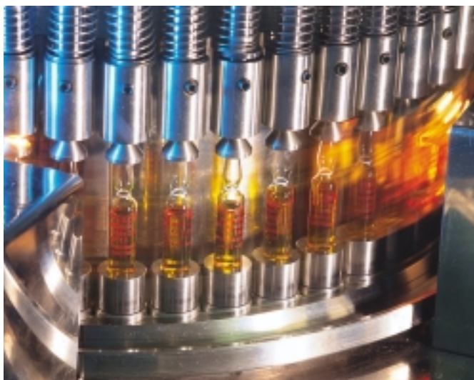
Electronic checking of injectable ampoules at the Ambarès facility.
