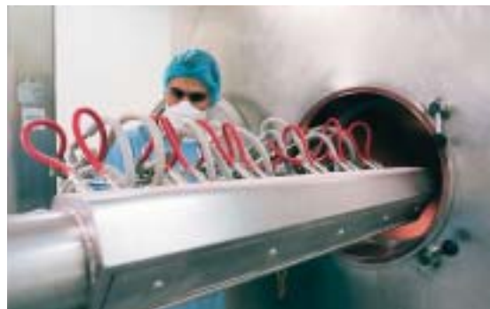
Coating: spraying nozzle ramp.
