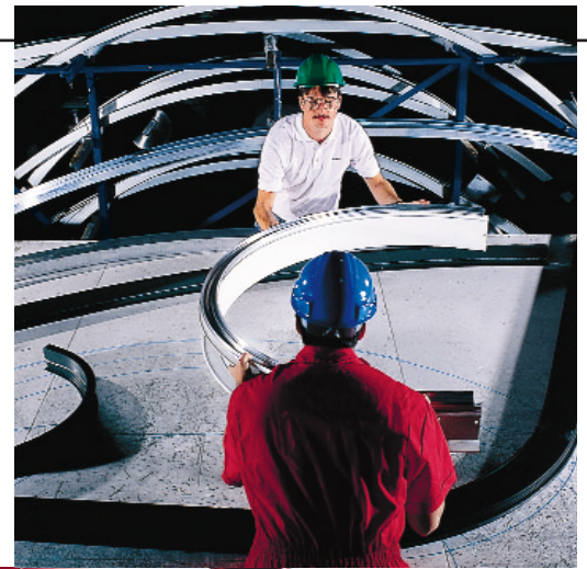
Keith Swankier (top) and Joe Allen stretch-forming architectural aluminum at Kawneer, part of the Alumax merger.
