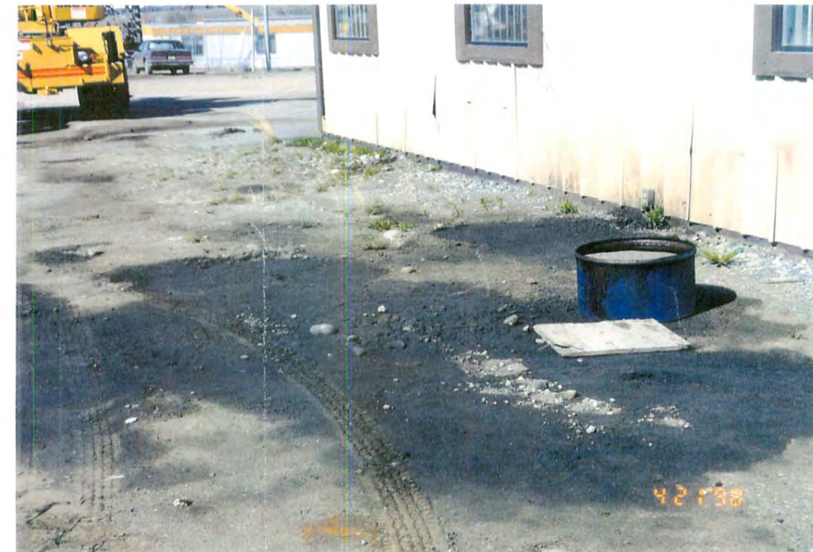
FIGURES 7 & 8: VIEWS OF A USED OIL SPILL NEAR THE SOUTHERN END OF THE FACILITY. THE MOST HEAVILY STAINED PORTIONS COMPRISE AN AREA EXCEEDING 250 SF, WITHIN A STAINED AREA APPROXIMATING 1900 SF.
