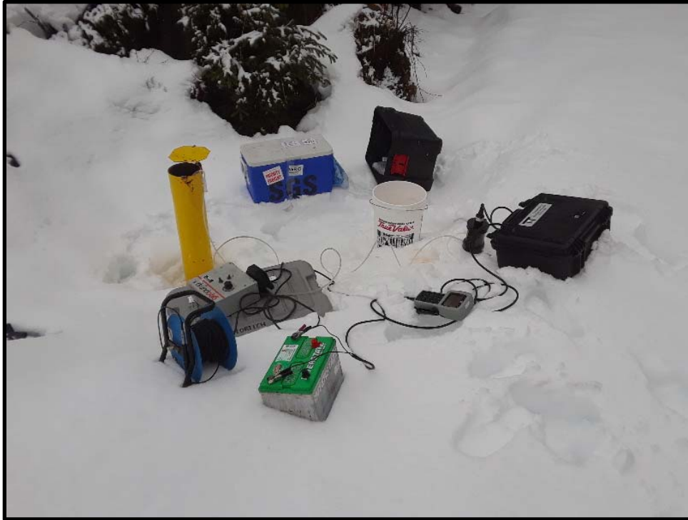
Photo 5: Looking south at MW-3 in DNR Pit #2 (Monofill Site) during well purging and water quality monitoring.
