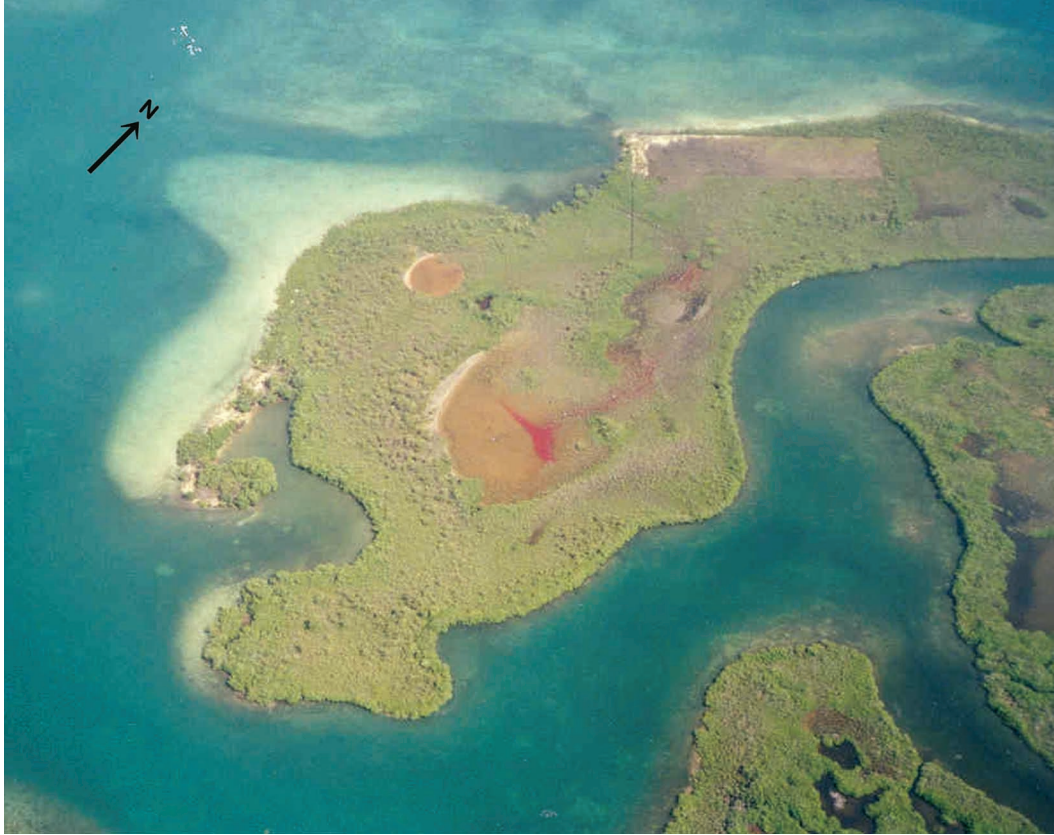
FIGURE 16. Aerial photograph of West Island looking to the northwest from an altitude of 600 m during the 5 June 1993 dye flow test, corresponding approximately to the time of run 4 of Figure 15. The dye is evident as the red configuration in the south pond.
