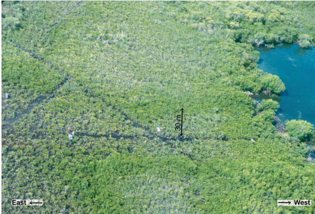
FIGURE 17. Aerial photograph taken in 1993 (looking south) showing survey lines that were newly cut in 1993. The original principal tidal flow path is evident as the darker green vegetation approximately 30 m south of the 1993 east–west survey line.
