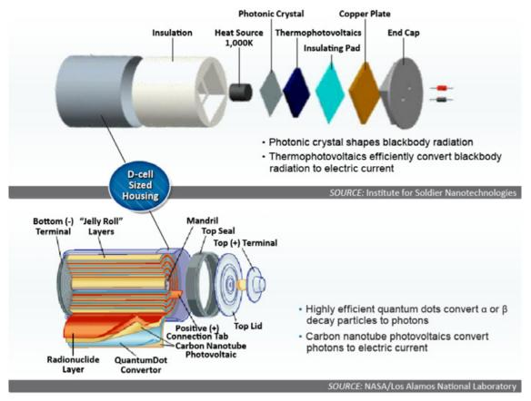
Figure 9 Radionuclide Battery Design Concepts
