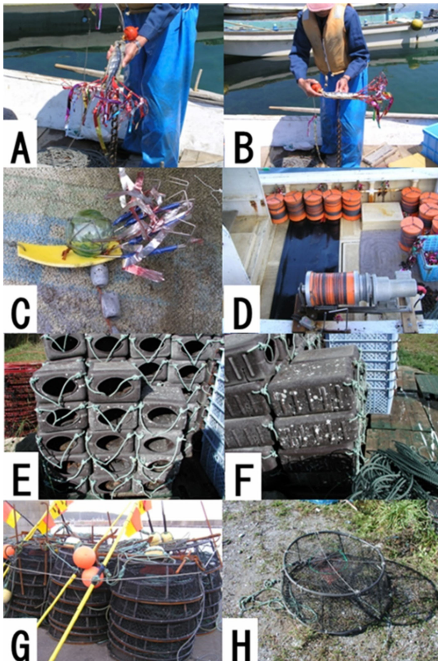
Figure 3. Japanese fishing gear for Octopus: Commercial gear used in Aomori and Hokkaido. (A–B) drag-line; (C–D) floating-barrel drift line (C: lure; D: stowed lure-barrel-line units); (E–F) octopus boxes; (G–H) octopus baskets. (Images: KN).
