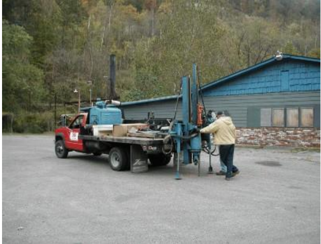
At left, a Geoprobe unit injects oxygen release compounds at a bio-remediation site. At right, a high vacuum pump truck extracts hydrocarbons.
