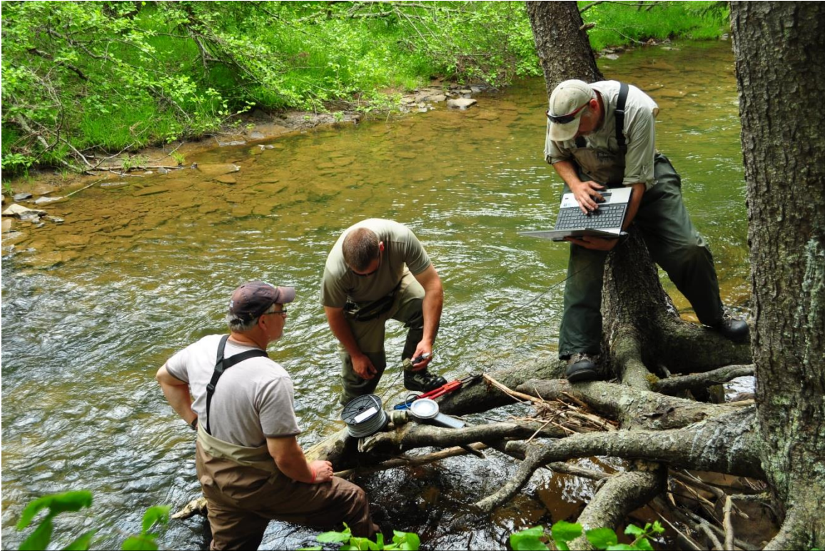
WAB staff installing continuous temperature and water level dataloggers in East Fork/Greenbrier River as part of U.S. EPA's Regional Monitoring Network for climate change studies.
