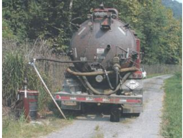
At left, a Geoprobe unit injects oxygen release compounds at a bio-remediation site. At right, a high vacuum pump truck extracts hydrocarbons.
