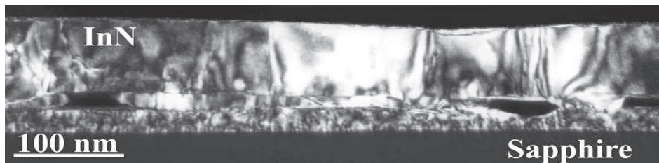
Figure 7.10: Transmission electron microscope image of a InN/GaN/sapphire sample. The three layers are recognizable by regions with different contrast. At the interface between InN and GaN it is possible to recognize voids of the size of several tens of nanometers.
