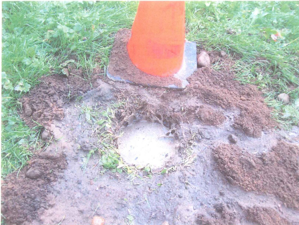
Legend 4. Water poured into holes to determine water permeability.
