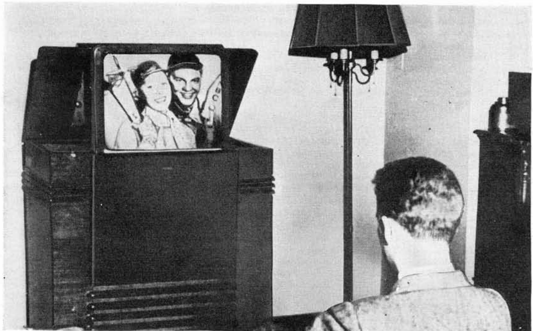
Large-screen television of 1939. The tube stands upright, projecting an image upward to a mirror on the slanting cabinet lid, from which it is reflected to the viewing screen.
